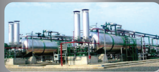
Oil Flash Vessel - OXY
