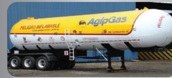
Auto-tank of 54 m3 for LPG - AGIP
